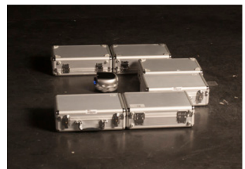
In a controls demonstration for one of Egerstedt’s online lectures, the Khepera III robot avoids hitting obstacles even as it slides close to them.
