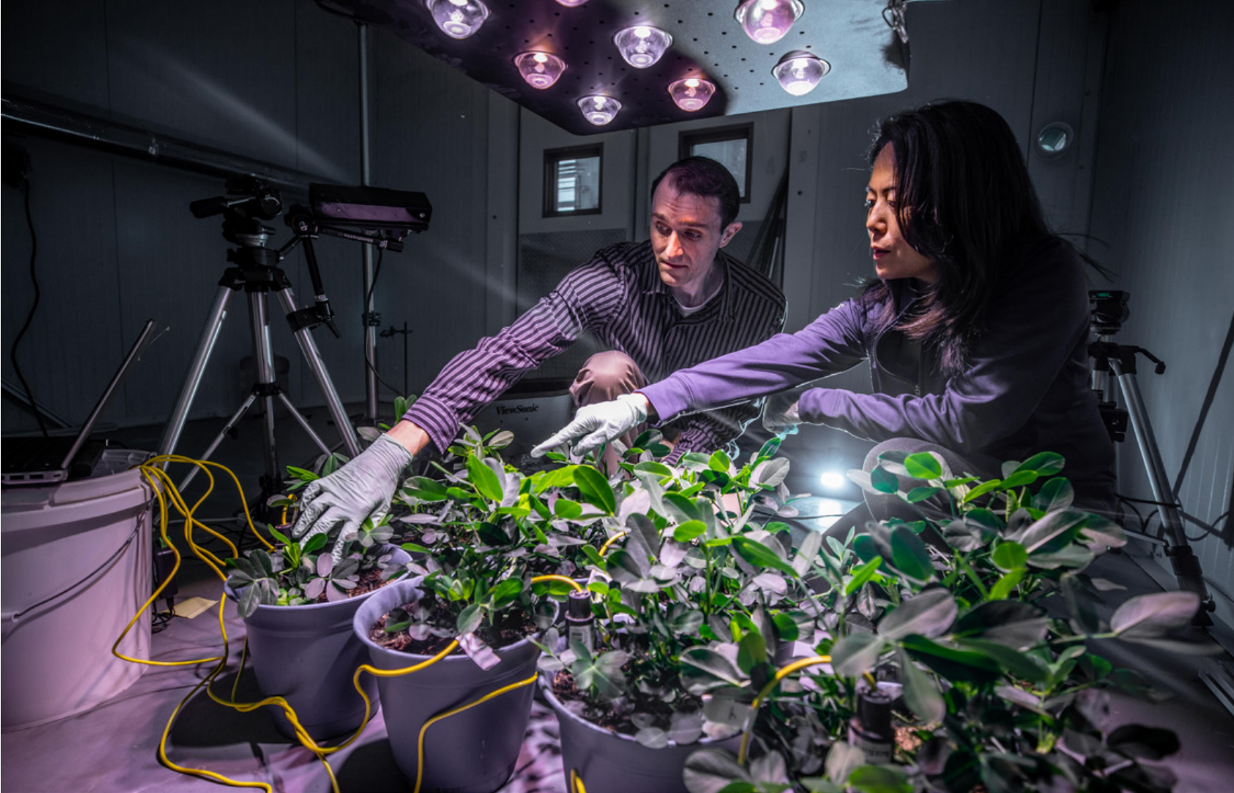
Above: Researchers Judy Song and Daniel Sabo install air sampling equipment used to collect volatile organic compounds from peanut plants. BRANDEN CAMP
